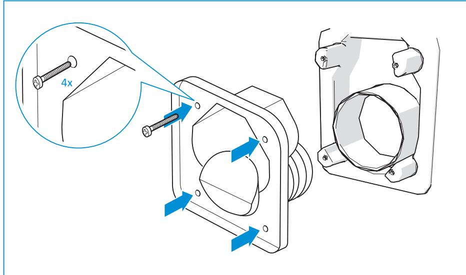
The required torque depends on parameters such as wall thickness, sealant, material and tools used. Therefore Thetford can only provide guidelines for the torque value.
